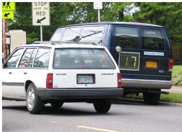
Figure 8. Mobile ASE unit with speed display board in Portland, OR
