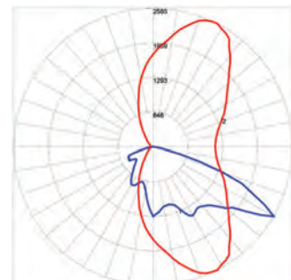
— Vertical plane through horizontal angle of maximum candlepower at 65° — Vertical plane through horizontal angle of 60°
