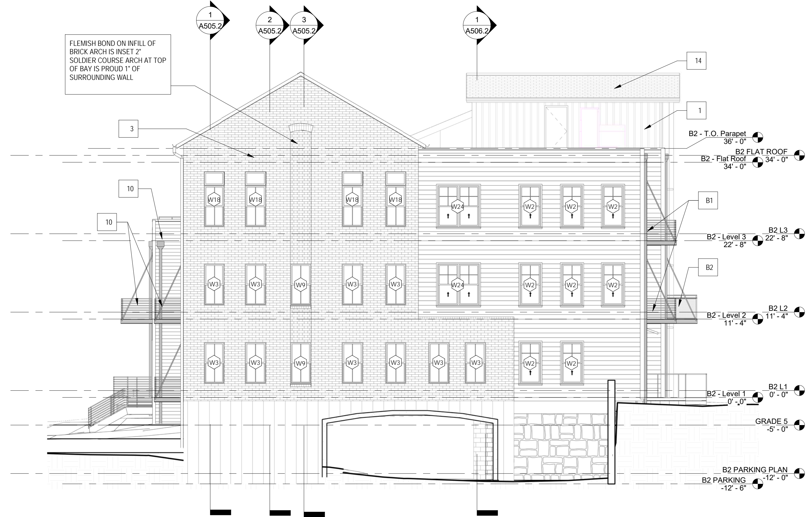
2 BLDG 2 - WEST ELEVATION A201.2 1/8" = 1'-0"
