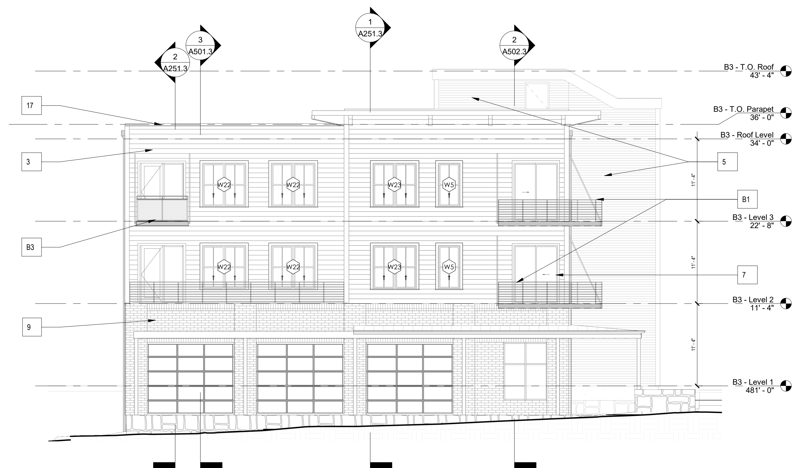
1 BLDG 3 - NORTH ELEVATION A200.3 1/8" = 1'-0"
